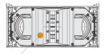
The frontal baffle's design increases the directivity of the line array doubling the radiation points on low/mid frequencies. The shape of the front baffle reduces the turbulence outside the waveguide decreasing the overall distortion.
