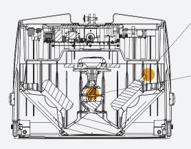
With its large format compression driver on a waveguide, the HDL 10-A offers superior intelligibility over distance.
