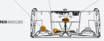
The custom 4PATH designed waveguide allows a precise coverage of 90 x 10 degrees, while also delivering a superb, linear high frequency response. The unique shape of the four ducts forming the guide creates an ideal isophasic load from 800 Hz to the highest audible frequencies.
